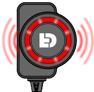
8 Flashing Red LEDs Vehicle battery voltage below 11.8v
