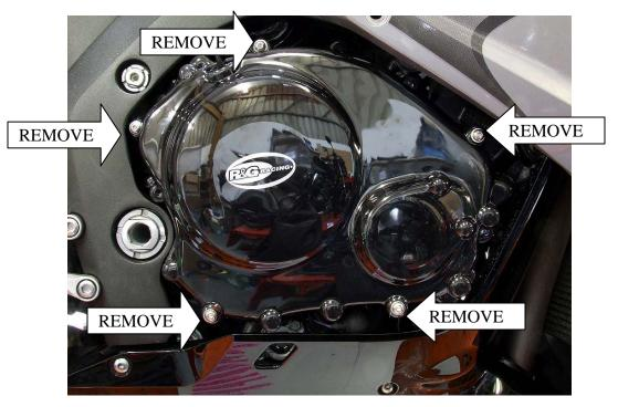
In this kit there should be: 1 x Engine Case Cover 5 x M6 button head bolts 5 x M6 washers 5 x black spacers 1 x 25mm length of heat shrink
