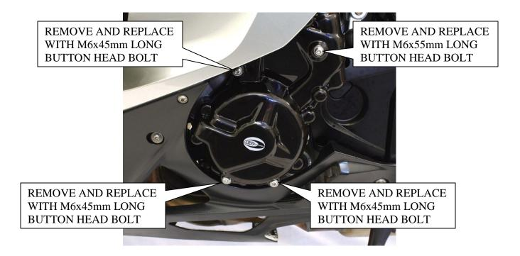
In this kit there should be 1 x Engine Case Cover (ECC0043) 1 x M6x55mm long button head bolt 3 x M6x45mm long button head bolts
