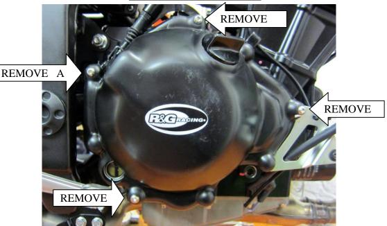
In this kit there should be: 1 x Engine Case Cover (ECC0140) 3 x M6x40mm long button head bolts 1 x M6x35mm long button head bolts
