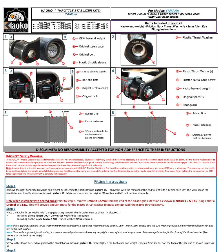
Attach the handguard to the Kaoko bar-end weight as shown in picture 3B and picture 4 using the original M8 \ bolt and steel washer.
